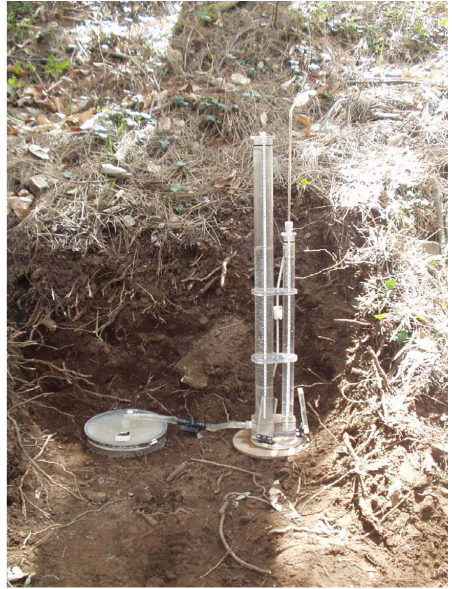
Disk infiltrometer : measures of hydraulic conductivities under depression (unsaturated conditions) – 3 sites, 3 depths in each site
