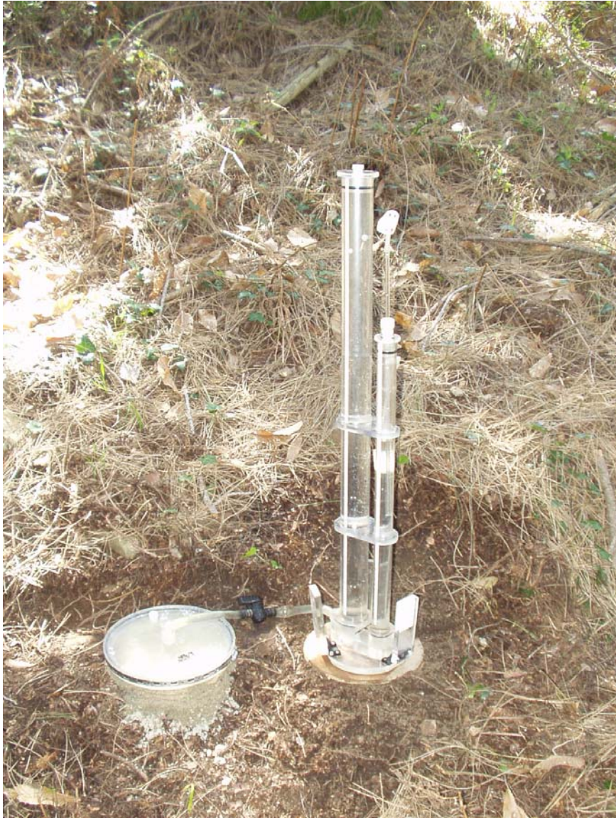
Disk infiltrometer : measures of hydraulic conductivities under depression (unsaturated conditions) – 3 sites, 3 depths in each site
